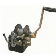
BOAT WINCH 3:1 FEATURES: • Includes light duty cable SPECIFICATIONS: • Maximum Weight Load: 500kg • Cable Length: 6m
