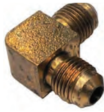
550-00634 SAE 450 FLARE BRASS FITTING, MALE UNION, 5/16 TUBE, 3/8 BSPT
